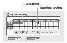
Each row of the grid is one day (you can set the timer recording for up to a month in advance). Each column is a 15 minute interval.
